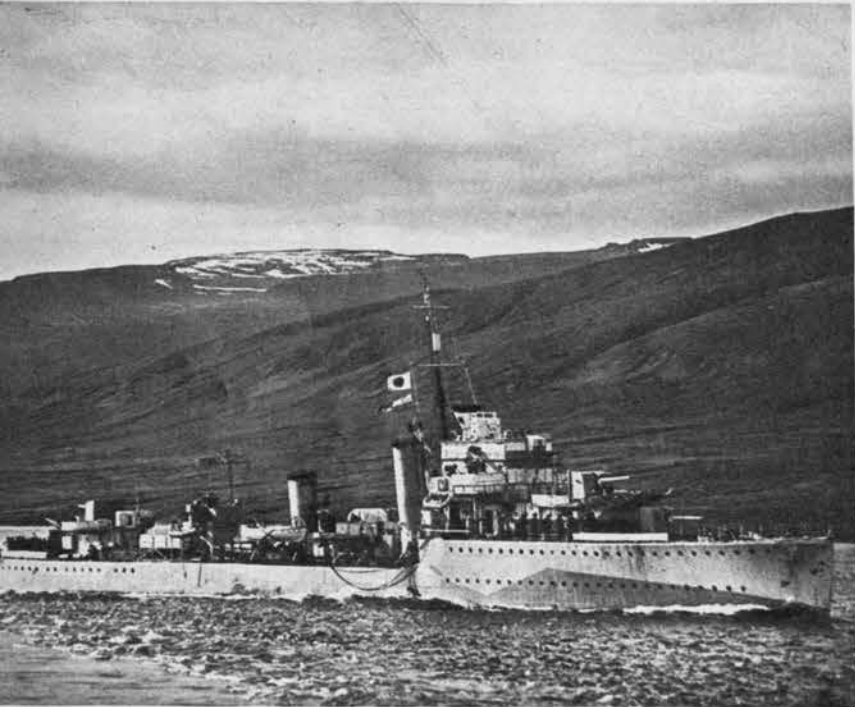
"A" AND "B" CLASS ships like Antelope (below) were first to mount their torpedo tubes in banks of four, to introduce box-shaped shields.
